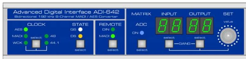
The **MATRIX** section is used to configure the routing of all inputs and outputs. Auto Delay Compensation (**ADC**) prevents offsets when using multiple ADI-642s.
