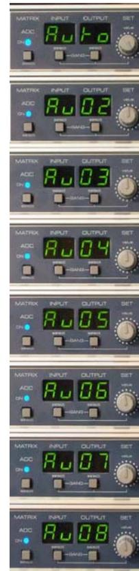
\* The ADI-642 uses the user bit of channel 19 to transmit the ADC and Auto Channel state to other devices.
