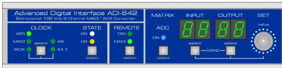
The ADI-642 can be remote controlled by MIDI commands. The button REMOTE is used to select the source of the MIDI remote control commands, and also the destination for the ADI-642's request replies. The standard MIDI ports or the MADi input and output can be chosen.
