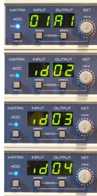
In Auto Channel mode the channel assignment is fixed and can not be changed. Therefore the buttons INPUT, OUTPUT and SET are locked on all ADC Slave units. The routing is as follows:
