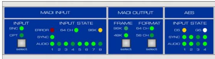
**MADI OUTPUT** is used to configure the MADI output as 56/64 channel or 48k/96k frame format.
