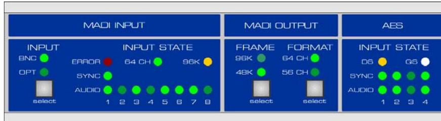
The MADi output signal can include 56 or 64 channels (FORMAT). The FRAME key switches the MADi output into native Double Speed mode (96K), in case internal or external clock allow this mode to be activated.
